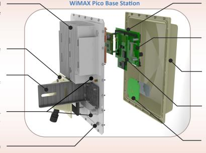
High Performance Motherboard with 533MHz Processor, 64MB SDRAM, and 16MB Flash
